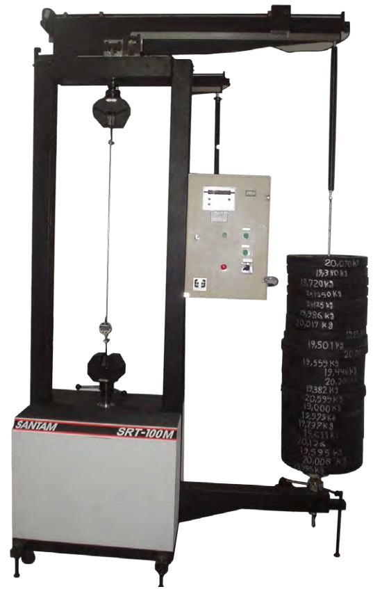
SRT-100M Dead Weight Loading Capacity 100 kN
