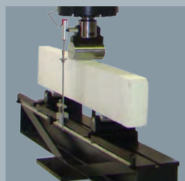
STD-1000 Universal Testing Machine Hydraulic, Closed Loop AC Servo Model with 3 Points Bending Fixture, C1609/C1609M – 12 Capacity 1000 kN
