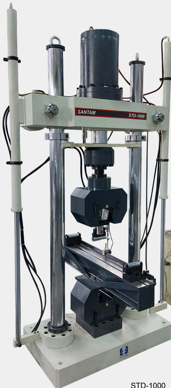
STD-1000 Universal Testing Machine Hydraulic, Closed Loop AC Servo Model with 3 Points Bending Fixture, C1609/C1609M – 12 Capacity 1000 kN
