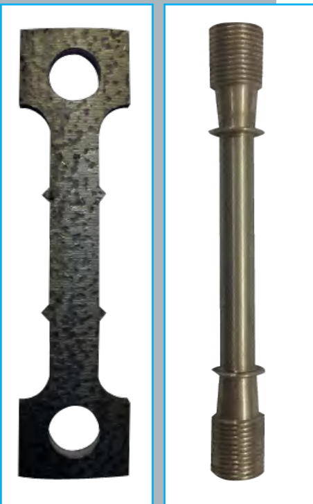
Pipe segment sample with Cuffs in the parallel length
