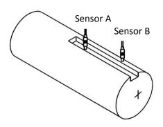
When rotation is in the forward direction, the notch is detected first by sensor A and then by sensor B. The notch must remain in view of sensor B.
