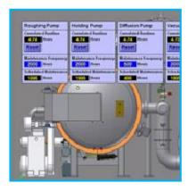
This system could be equipped with an intuitive and easy to use computer interface, allowing full control of the furnace. In addition it provides data trends and storage (Data acquisition), display and logging of alarms, unlimited recipe profiles temperature control, security, etc.
