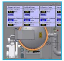
This system could be equipped with an intuitive and easy to use computer interface, allowing full control of the furnace. In addition it provides data trends and storage (Data acquisition), display and logging of alarms, unlimited recipe profiles temperature control, security, etc.
