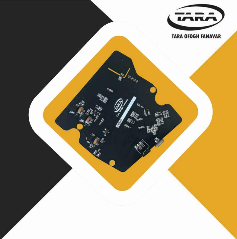
The D1304-01 driver circuit is a powerful hardware module, developed for TCD1304, Toshiba CCD linear image sensors. The circuit takes the advantages of FPGA as the core microprocessor. A 16-bit A/D converter analog signal processing circuit allows users fast data processing. The circuit transfers data to PC and controlled from the PC by a USB Micro 2.0 connector. D1304-01 is compact, lightweight, and easy to handle driver.
