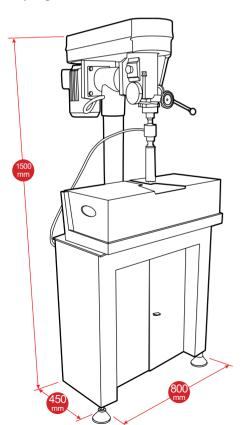
variety of Dimond-tipped coring bits, which allows the user to prepare core specimens varying from 0.5ò to 5ò in diameter. Water cooling system permits rapid and efficient cutting without damages to the bit and the machine, and includes a water pump, water tank, flexible hose, water swivel, and drinage tray. It provides core specimens for Routine and other tests frequently conducted in petroleum reservoir research facilities.
