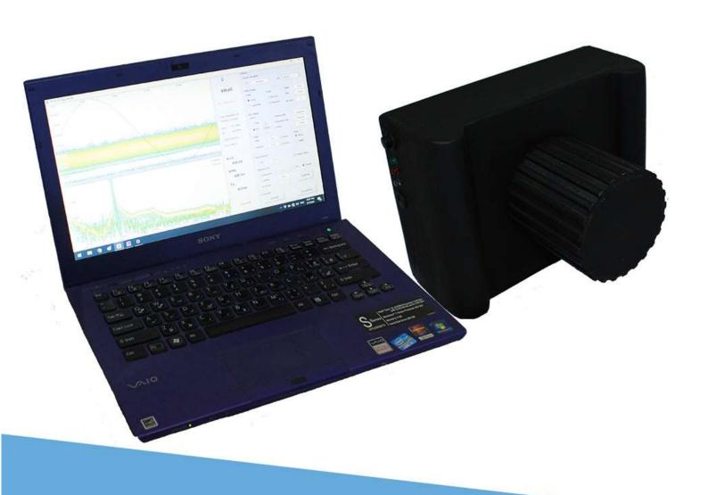
Using PDCam, PD measurement is faster, more accurate and more effective than ever before.
