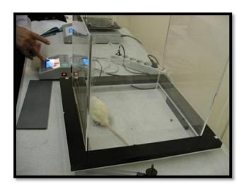
In order to obtain qualitative analysis of mouse or rat home cage activity with Photobeam Activity System. The subject's locomotor activity will be precisely tracked by a 5×5 photobeam configuration for mice or a 2×2 photobeam configuration for rats that reports breaks in real time, requiring no special calibration. Test up to 6 stations at a time and set it all up quickly with no technical knowledge required.
