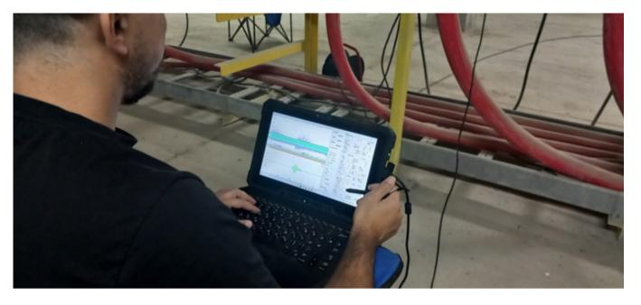
**PDCAM** is a handheld Online Partial Discharge Monitoring System for use on HV and MV cables, terminations, joints, switchgears and rotating machines. Its weight is light but can handle heavy duties. it offers real time PD acquisition on using different partial discharge sensors.
