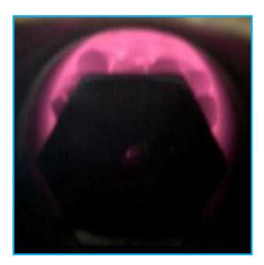
The main advantage compared to VRFs is no contamination between the materials inside the furnace and the heating elements.
