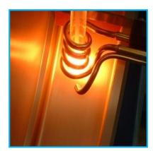
Standard versions of the melt spinners are delivered with boron nitride crucibles; quartz crucibles are available on demand.
