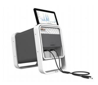
The development of portable Raman spectrometers has drastically changed the way the industry conducts quality control for incoming raw materials. Raman has always provided advantages over other methods in that it does not require sample pre-treatment or direct contact with the sample, and has the unique capability of being able to test a sample directly through a transparent packing material like glass or plastic.
