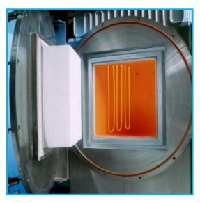
Other possibilities include the heat treatments of metals, crystal growing and the manufacture of ceramic powders. Hydrogen processes are limited to 1000°C. Vacuum operation is only recommended in low vacuum ranges.
