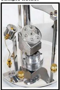
The DSR1 can be equipped with different sample stage configurations depending on the user requirements. The sample stages are rotatable with adjustable height and can be changed easily.
