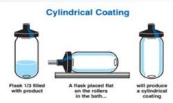
Fill the flasks slightly less than 1/3 and place the flask on the rollers. The rollers will rotate the flasks while the refrigerated bath freezes the product. This results in a thin, even, high surface area coating of frozen material on the inside of the flask.
