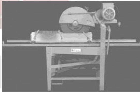
The standard electric motor is 220 VAC, 60 HZ, and single phase. The saw assembly is 70 cm high, 65 cm wide, 120 cm long and weighs 120 kg. Includes a core guide and clamp assembly for holding core for smooth slabbing operation. Liquid coolant pump included for fluid recirculation.
