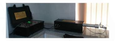
Optionally, a computer data acquisition and supervision system can be provided. Furthermore, a variable temperature heating mantle can be supplied to heat the fluid up to 150°C. These pumps can be customizes based on the client requirements. For example, although standard material for wetted parts and volume are stainless steel and 500 cc, hastelloy can be requested for corrosive fluid applications and diffident volumes can be ordered.
