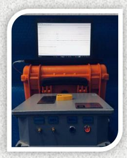
The ART-AR243 is a three channels accelerometer which record acceleration through the x,y and z axis.
