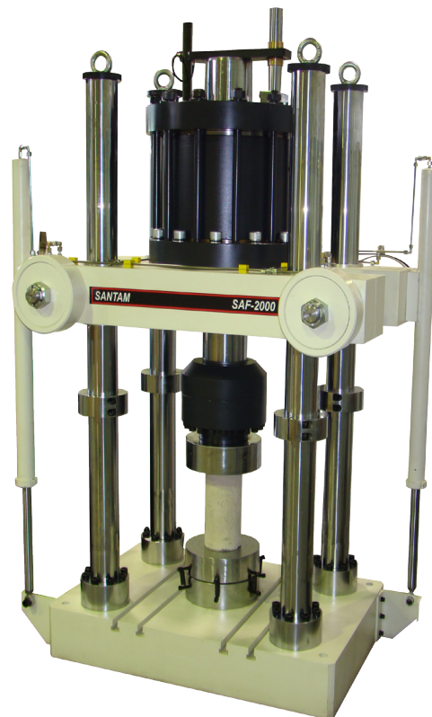
SAF-2000 with Compression Platens Self Align
