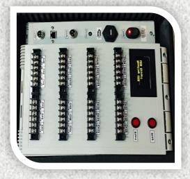
The ART-SR2424 is a multi-channel seismic recorder for reflection, refraction and exploration seismic investigations.
