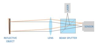
It is basically composed of a collimator and a telescope, combined by a beam splitter. The former projects a parallel beam, while the later images the reflection onto the sensor.
