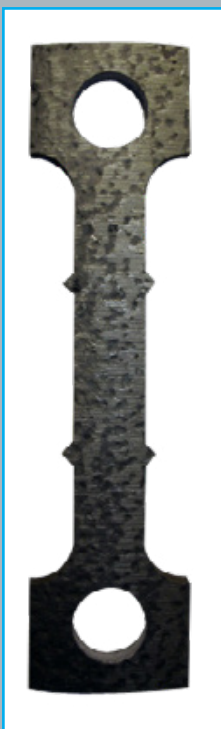
Pipe segment sample with Cuffs in the parallel length
