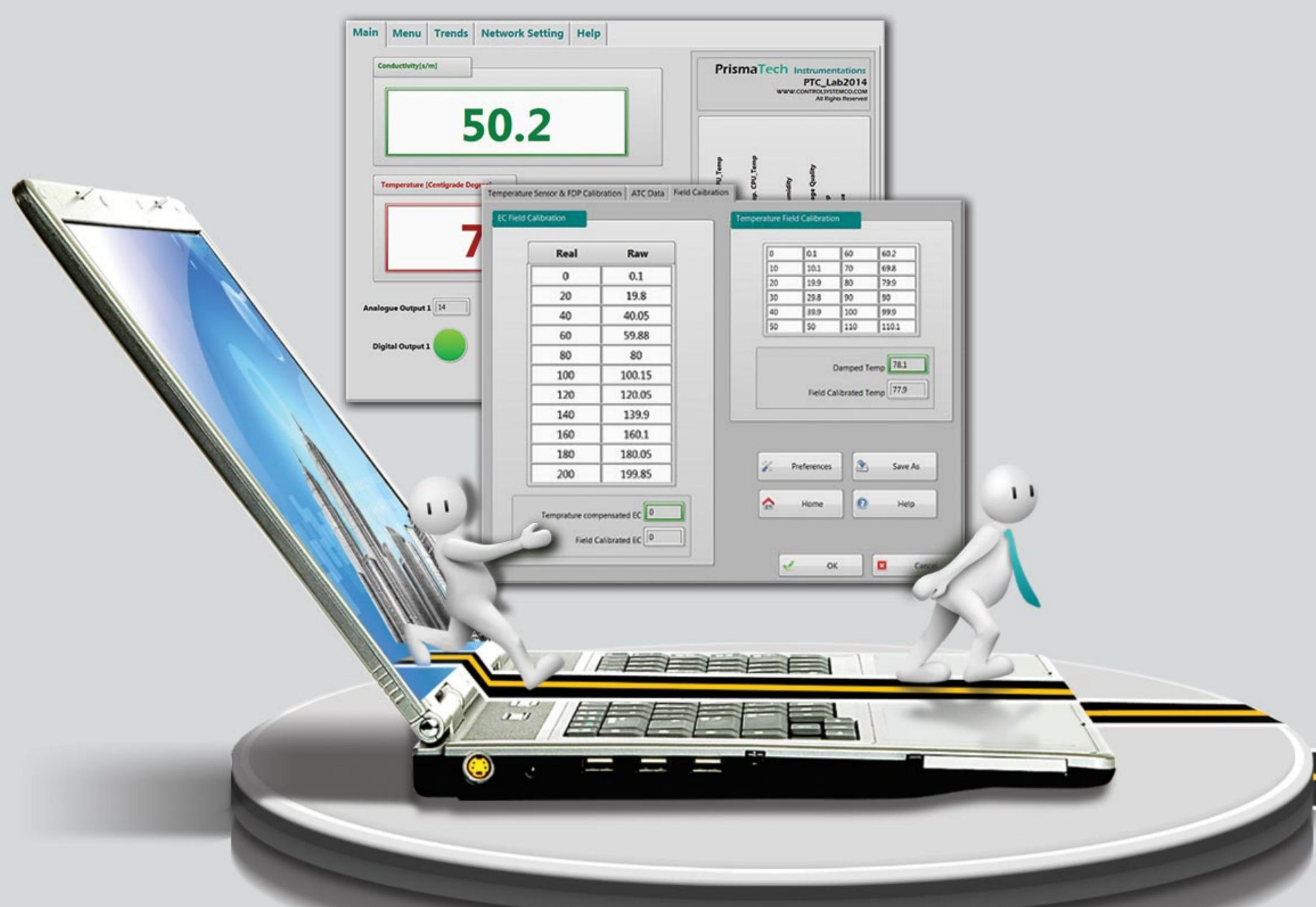
PrismaTech® Inline Conductivitymeter in addition to measuring the conductivity of the solution is capable of control the conductivity of the process simultaneously by the aid of two analog current outputs (0/4-20mA PID Controller), one digital input and two digital outputs without the need for any other separate control equipment.
