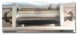
between the flow distribution plugs and the core sample. Special Viton sleeves with two embedded circumferential electrodes are employed for high-accuracy sample resistivity measurements. Two other electrodes are in contact with the electrically isolated distribution plugs, thus allowing both two and four point resistivity measurements.
