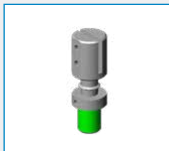
TF1000-20P3C High Temperatur Tensile Test Adaptor (for sheets) t=3-5mm 1000°C capacity 20 kN
