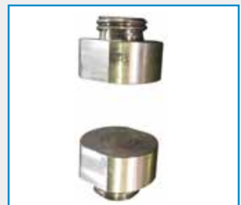
CF1000-20P24 High Temperatur compression Test Adaptor \phi=20 mm 1000°C capacity 20 kN
