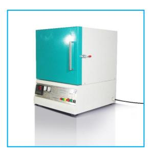
proper sealing could be utilized. Working temperature of up to 1250, 1450, 1600, 1700 and 1800°C are available.
