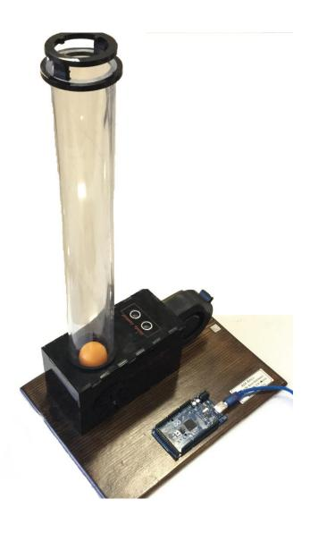
The AB\_HILS is a Hardware In the Loop Simulation system for student to understand how to design and implement a real-time embedded control algorithm rapidly. In this experimental setup the height of a ball is stabilized by speed control of a DC fan. The fan blow the air in a tube to overcome the gravity of the ball. A set of IR and ultrasonic sensors is used to measure the height of the ball and define the desired level of the ball.
