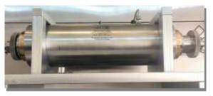
between the flow distribution plugs and the core sample. Special Viton sleeves with two embedded circumferential electrodes are employed for high-accuracy sample resistivity measurements. Two other electrodes are in contact with the electrically isolated distribution plugs, thus allowing both two and four point resistivity measurements.
