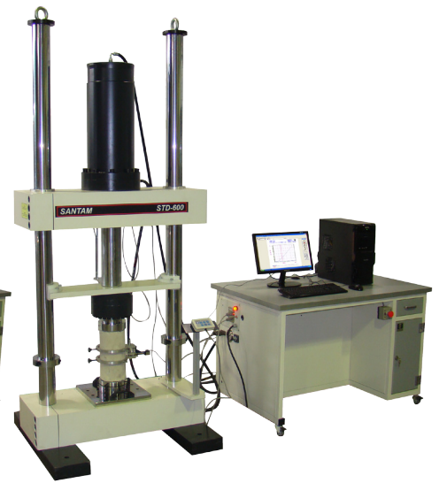
STD-600 With Compression Platens Self Align
