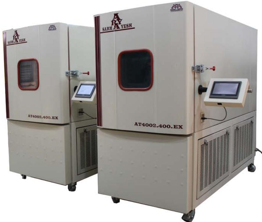
Explosion proof temperature test chambers
