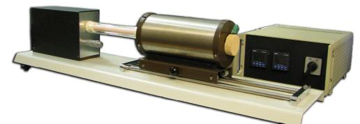
DAMA Pajouh Arvin Dilatometer 101 is a complete, compact, easy to use, bench top system comprised of furnace (for variety of temperature range, including sub-ambient); a sample holder system fused silica or high alumina); a control / sample thermocouple; a sample displacement measuring system (probe rod and LVDT sensor); furnace controller data acquisition system (stores temperature and displacement data)
