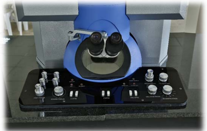
↑ ARA-TEM main control unit panel
