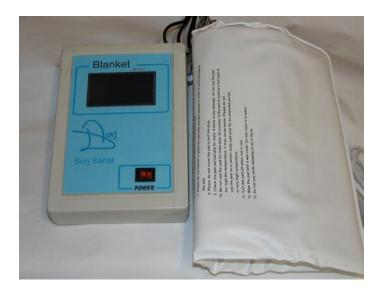
The temperature Controller monitors and controls the body temperature of rats and mice. This microprocessor-based instrument provides heating using a resistive heating blanket. An LCD panel displays the current body temperature and the targeted set-point temperature. Rat body temperature is measured real time using a rectal probe connected to the microprocessor. After plugging in the probe and heating blanket, the animal's temperature is shown on the display.
