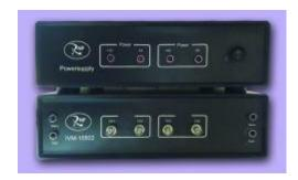
1 Voltage Measurement input: range: 15V, Resolution: 0.1mV\*2 Programmable Voltage Outputs:\* range: 15V, Resolution 1mV Sampling rate: 10 Sample/Sec\*IVM-50:\*1 Current Measurement input: \* range: 100mA, Resolution: 1nA
