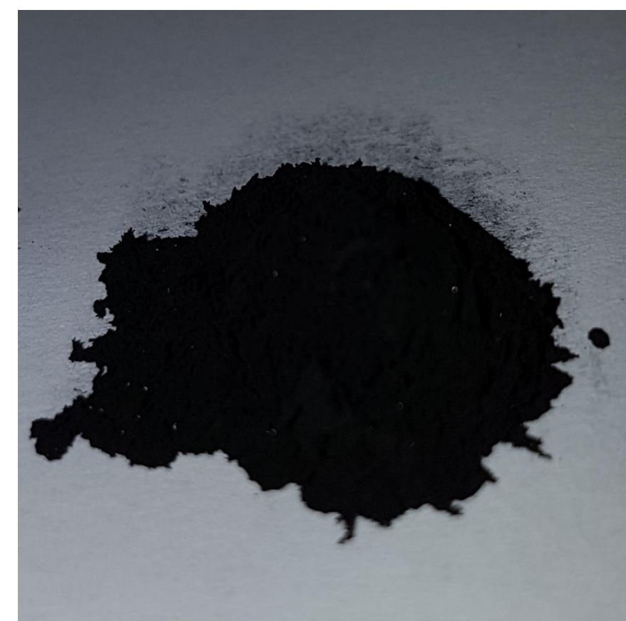
Image of iron(II,III) oxide nanopowder (FNP201)
