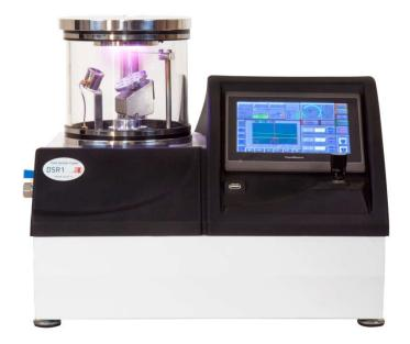
The Desk SEM Coater model DSR1 is a compact coating system able to coat noble metals such as gold (Au), palladium (Pd), platinum (Pt) and gold/palladium (Au/Pd) thin films on non-conductive or poorly conductive specimens. Uniform thin films with fine-grain sizes are formed in a fast cycle time. The produced thin film is suitable for scanning electron microscopy (SEM) analysis.
