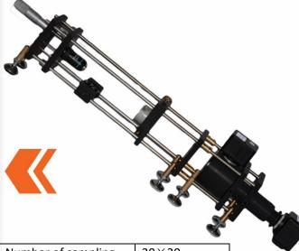
Number of sampling20×20Sampling Pitch140 μmEffective focal4 mmWavefront Accuracy20 mm
