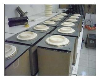
This division has one of the most advanced winding machines in the world, so this capability enables us to manufacture high energy pulse discharge capacitors with **internal series configuration**. This type of winding not only decreases the inductance, but also increases output current capability and mechanical strength.
