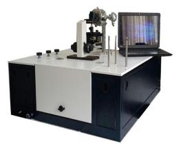
precipitation is determined through visual observation of formation of solid particles in the fluid. Subsequent studies regarding physical change of solid particles and/or effect of inhibitors can be hold by the versatile apparatus.
