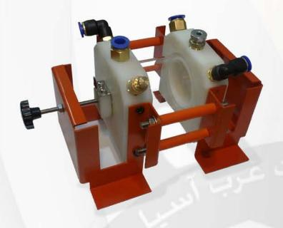
Corrosion Cell **Model FGS-300** offered by RGS Co. suitable for experiments conducted under ambient to 80C by use of heating elements. Due to its high sealing conditions, this product is also appropriate when gas purge is required.
