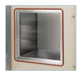
Yaran Vacuum Ovens are equipped with silicone gaskets. While these gaskets resist a wide variety of temperatures and pressures, they can breakdown in the presence of solvents and acids. For solvent applications we recommend using the Buna M gaskets, and for acidic applications the Fluorosilicone gaskets.
