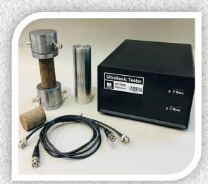
The ART-UST-PC is a precise laboratory instruments which measures ultrasonic wave velocity in asphalt, soil, rock, ice & concrete specimens.
