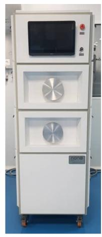
of course with higher costs. The SI-LP80 is a unit which has been designed with a novel "double-wall" stainless chamber to ensure about the safety of the system, once exposed to hazardous gases such as hydrogen and silane. A dual-pumping system allows achieving excellent conditions for the formation of suitable layers.
