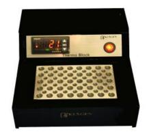
The block is made of an aluminum alloy with excellent thermal conductivity and has different hole sizes for 1.5 & 0.5 ml microtubes..
