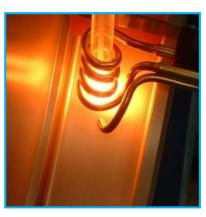
Standard versions of the melt spinners are delivered with boron nitride crucibles; quartz crucibles are available on demand.
