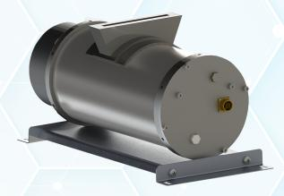
**RAXON200HPO** is a high-power industrial X-ray source for producing a beam of high intensity X-rays with small focal spot and high stability which ensures uniform beam intensities and dose rate throughout its fan-shaped beam. Stable voltage and electrical power applied to X-ray tube guarantees stable dose exposure and high-quality images in digital radiography systems.
