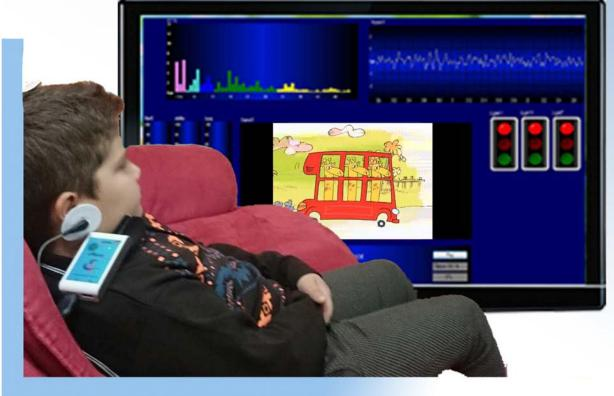
The eWave is a small and high-tech system for recording EXG (EEG, ECG, EMG, EOG, ERG) signals in Biofeedback and neurofeedback applications.
