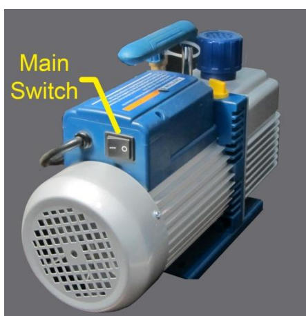
Figure 4-3: Rotary Pump Main power Switch
